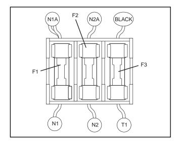
Figure 8. Fuse Holder and Fuses
